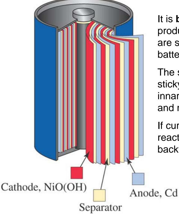
It is **because** the products of the reaction are solids that the Ni-Cd battery can be recharged
