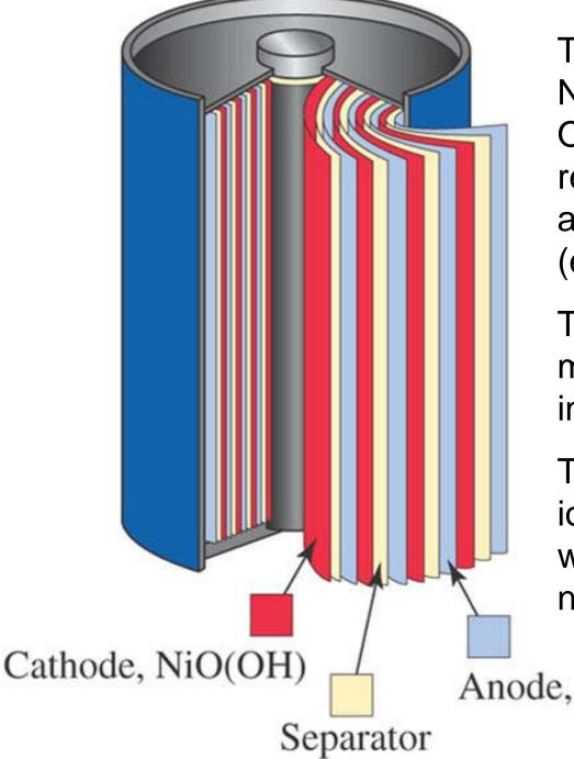
The cell contains a paste of NaOH – this provides the OH<sup>-</sup> ions needed for the reaction, while also providing a medium to pass charge (electrolyte)
