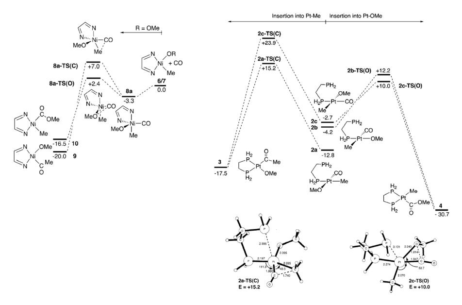
Computed reaction profiles (in kcal/mol) for the migratory insertion reaction CO. Energies are relative to the starting complex + free CO set to zero.
