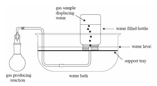
Calcium carbonate (CaCO<sub>3</sub>, molar mass 100.1 g/mol) is heated in the flask, and decomposes to form CO<sub>2</sub> gas according to the following reaction:
