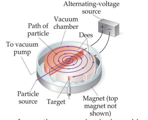
Nuclear transformations can be induced by accelerating a particle and colliding it with the nuclide in particle accelerators called cyclotrons or synchrotrons or *particle smashers*.
