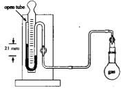
The mercury height in the outer arm is higher than that of the inner arm by 21 mm. The barometric pressure in the laboratory is 752 mm Hg. What is the pressure of the sample gas in atmospheres?
