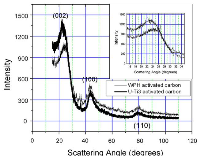
Fig. 3. XRD for WPH and U-Ti3 activated carbon. The enlargement of (0 0 2) peaks and fittings are shown in the inset.
