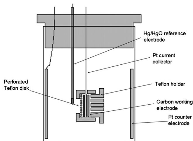
Fig. 1. Electrochemical cell used in the experiments.
