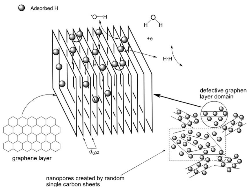
Fig. 6. Illustration of H electrochemical insertion into interlayer structure of microdomain of graphene layers.
