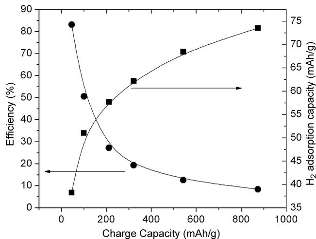
Fig. 7. Discharge and charge efficiency for hydrogen insertion. The electrode was made with M1470 activated carbon. The electrode was charged (reduction) at  $100 \text{ mA g}^{-1}$  current density and discharged (oxidation) at  $50 \text{ mA g}^{-1}$  current density. The efficient was defined as the percentage of oxidation capacity against reduction capacity.
