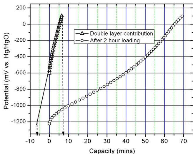
Fig. 2. Discharge of stored hydrogen, double-layer contribution.
