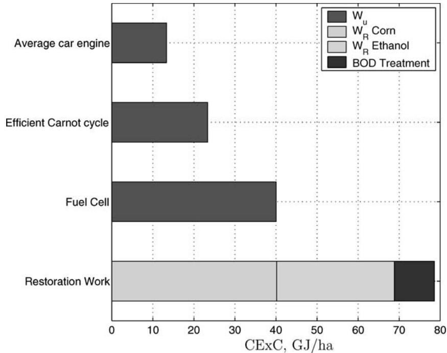
**FIG. 42.** The minimum cumulative exergy consumption by the industrial corn-ethanol cycle and its maximum useful work,  $W_u$ . For comparison, the cycle's ethanol is burned in an average car engine, an efficient Carnot engine, and in an ideal fuel cell. This comparison demonstrates that the industrial corn-ethanol cycle is unsustainable by a factor of 100–600%. It seems no adjustment of process parameters will change this terrible situation.
