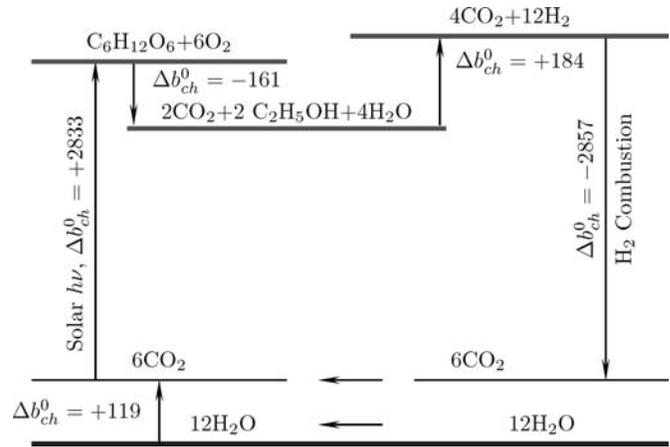
FIG. 39. Exergy diagram of the ideal CO<sub>2</sub>-Glucose-EtOH-H<sub>2</sub> cycle.
