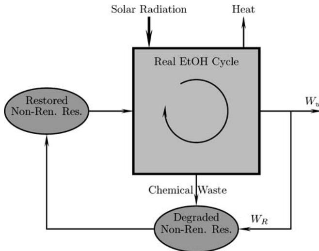
**FIG. 40.** A part,  $W_R$ , of the useful work,  $W_u$ , from the industrial corn-ethanol cycle is diverted to “undo” mining of the environment by this cycle. If  $W_u > W_R$ , there is net benefit from the ethanol biofuel, otherwise its use should be stopped.
