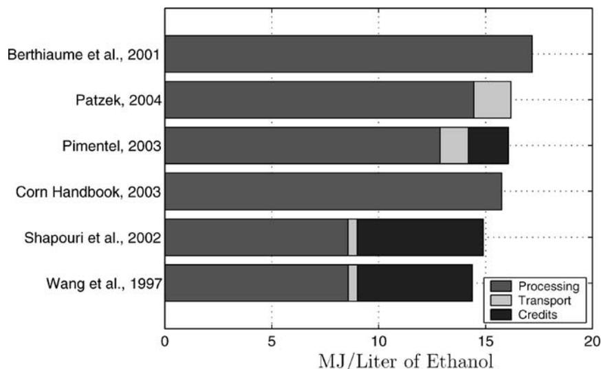
**FIG. 15.** The average fossil energy inputs to ethanol production in a wet milling plant. The length of each bar is the total energy outlay to produce 1 liter of EtOH, and the black (rightmost) parts denote the size of energy credits assumed by the different authors.
