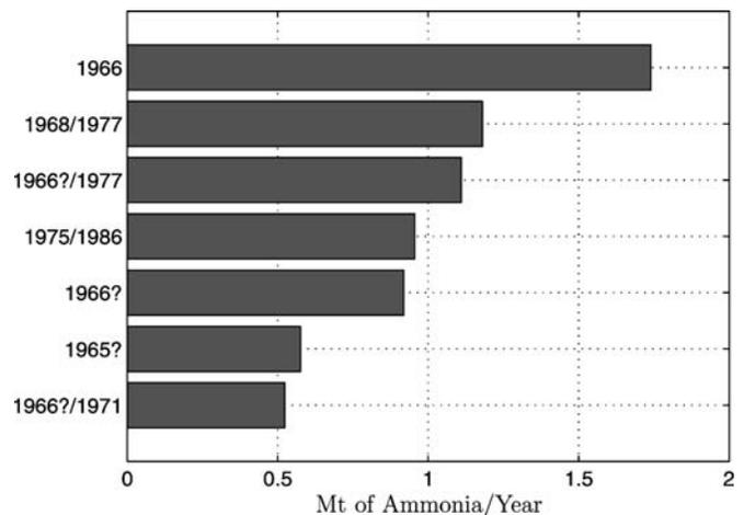
FIG. 2. Together, these seven largest plants produce 40% of the U.S. ammonia. The first dates refer to plant opening. Some of the plants were later expanded and revamped, as indicated by the second dates. Source: Ernst Worrell *et al.* (2000).
