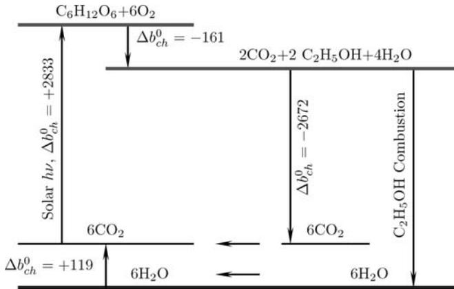
FIG. 38. Exergy diagram of the ideal CO<sub>2</sub>-Glucose-EtOH cycle.
