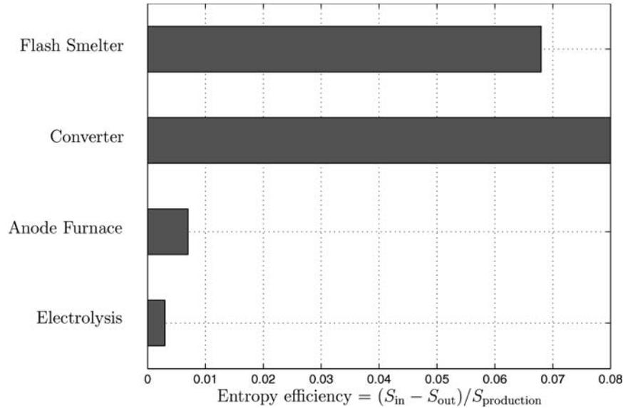
**FIG. 20.** The Second Law efficiency of copper production is incredibly small. The steps in sorting the copper atoms are: Ore Concentration 2% → 30% Cu (not shown); Smelter 30% → 63% Cu; Converter 63% → 99.1% Cu; Anode furnace 99.1% → 99.55% Cu; and Electrolysis 99.55% → 99.99% Cu. Source: Stefan Gössling, *Entropy Production as a Measure for Resource Use*, University of Hamburg, 2001.
