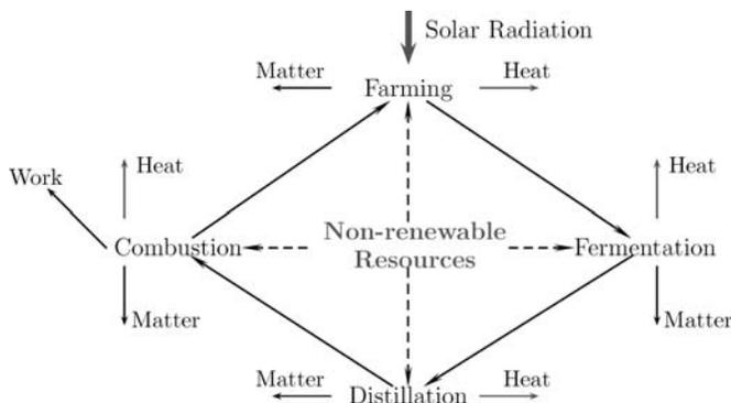
**FIG. 33.** The industrial corn-ethanol cycle. The nonrenewable resources (NRRs) at the center of the cycle are: crude oil, methane, coal, electricity from fossil fuels, earth minerals, soil nutrients, groundwater, and so on.
