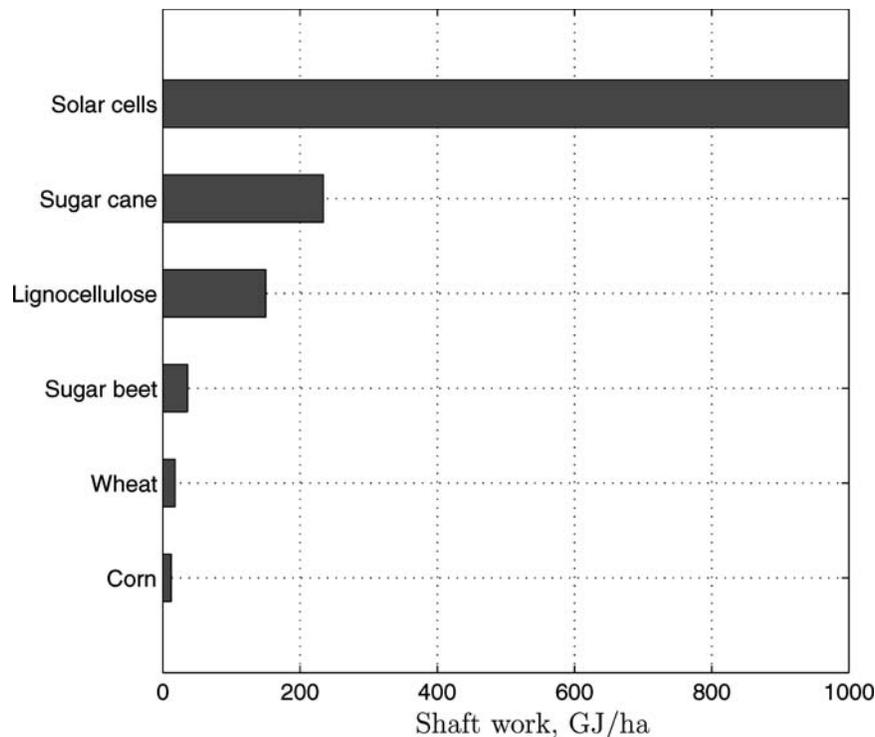
**FIG. 45.** Shaft work obtained in 120 days from the solar cells on 1 ha dwarfs that from the ethanol produced from all major biofuels. The *maximum* ethanol biofuel energy yields are from Table 7, p. 28, in Hamelinck' Ph.D. thesis (2004). The conversion efficiency from ethanol to electrical shaft work is an optimistic 0.6. The *minimum* solar cell yield follows the assumptions in this appendix. Note that annually the solar cells produce ~100 times more electricity than corn ethanol.
