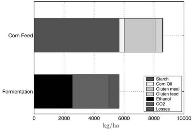
FIG. 13. The result of practical corn conversion into ethanol is 0.372 L EtOH/kg dry corn grain = 2.50 gal EtOH dry bushel = 2.18 gal EtOH wet bushel with 15% moisture.
