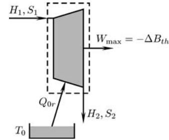
**FIG. 29.** Exergy balance in an isothermal, ideal flow machine. The maximum possible shaft work from this machine is equal to the negative change of thermal exergy.
