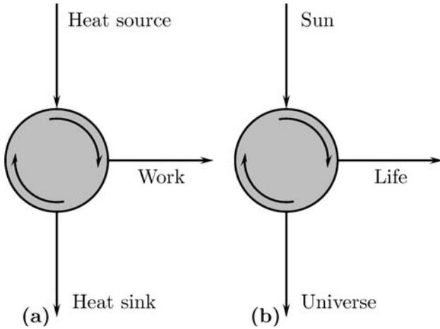
FIG. 28. Thermodynamic cycles: (a) A heat engine, and (b) An ecosystem.
