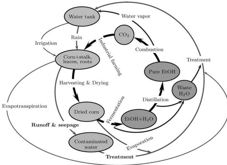
**FIG. 37.** The water cycle in corn-ethanol production. Compared with the water requirement by corn plants, the feed water requirement of an ethanol-producing plant is small, and the link between the tank and the fermentation stage was not drawn.
