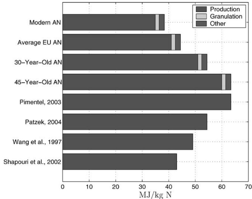
**FIG. 3.** The various estimates of the unit energy consumption to produce ammonium nitrate (AN). The estimates by Shapouri *et al.* are listed in Shapouri *et al.* (2002), by Wang *et al.* in Wang *et al.* (1997), and Pimentel's (2003) estimate of 78.1 MJ/kg N was adjusted down to the 45-year-old AN.
