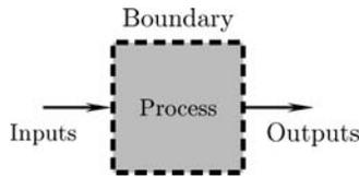
FIG. 19. The *boundary* separates the process from the environment at any time (it is the *interface*), and it defines the *duration* of the process. A process *may not* be describe by what happens inside or outside of it, but only by what crosses its boundary.
