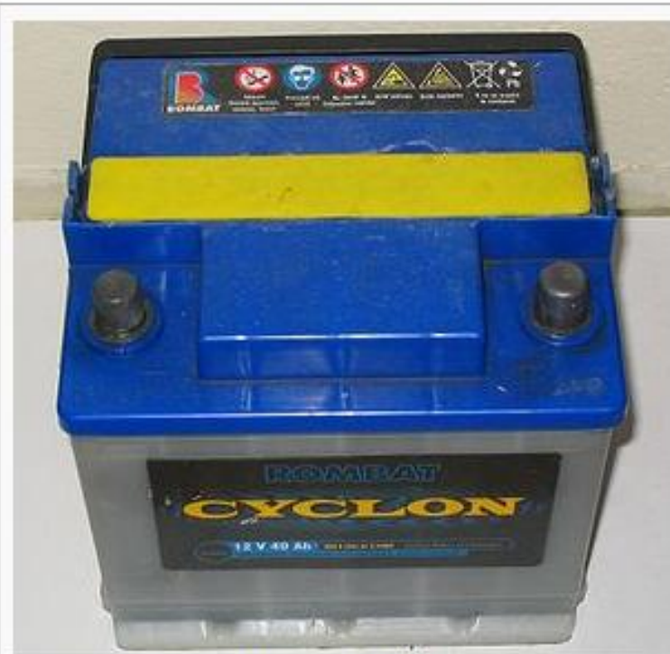
lead acid car battery
