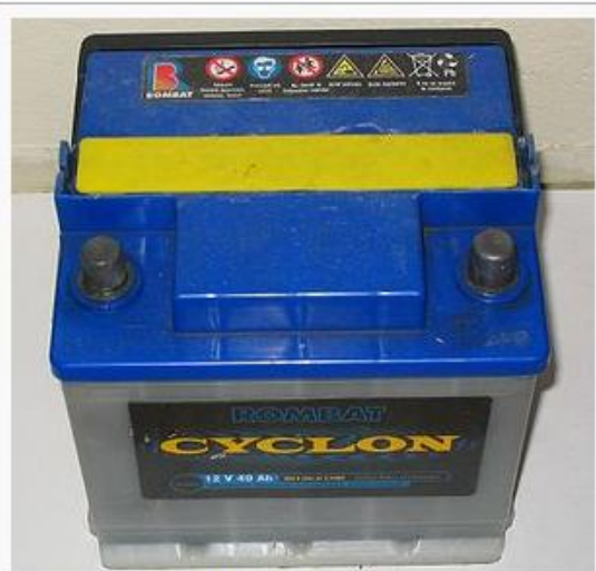
lead acid car battery
