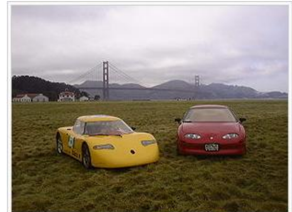
The tzero on the left can go up to 300 miles (480 km) at 70 mph (110 km/h) using Li-ion batteries, while the EV1 on the right has a range of 160 miles at 65 mph using NiMH batteries, or 80 miles (130 km) with lead acid ones.
