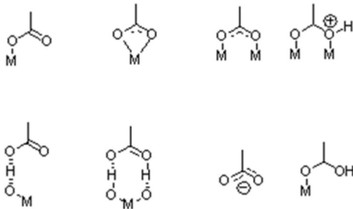
Possible binding modes for a carboxylic acid anchoring group at TiO<sub>2</sub> (M = Ti)
