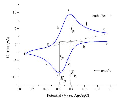
Fig. 1: Cyclic voltammogram of ferrocene reported vs. Ag/AgCl in 0.1 M Bu<sub>4</sub>NPF<sub>6</sub> acetonitrile electrolyte ( $E^{o'} = 0.45$  V). *ohmic ocurrent*
