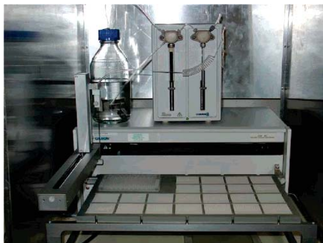
Figure 4. Autosampler with custom-made MTP/silica gel plate holder. An HPLC needle is mounted on the XY arm at the left and is connected to the washing pump (center). The needle takes 30 \mu L from one of the MTP wells, distributes 1 \mu L onto each of the 22 silica gel plates, and goes to a washing cycle before resuming distribution with the next MTP well.
