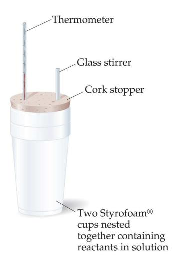
Because the specific heat for water is well known (4.184 J/mol-K), we can measure  $\Delta H$  for the reaction with this equation:
