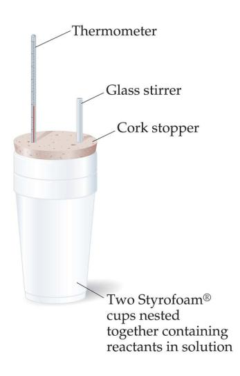
By carrying out a reaction in aqueous solution in a simple calorimeter such as this one, one can indirectly measure the heat change for the system by measuring the heat change for the water in the calorimeter.
