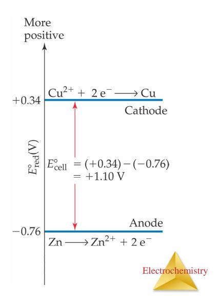
A voltaic cell is based on the following two standard half-reactions:
