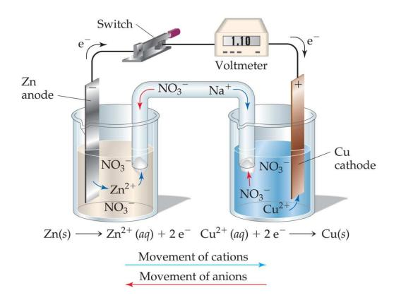
Once even one electron flows from the anode to the cathode, the charges in each beaker would not be balanced and the flow of electrons would stop.
