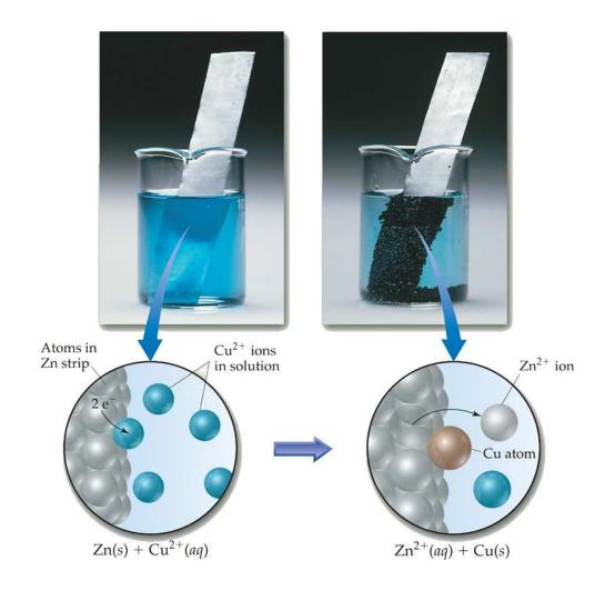
In spontaneous oxidation-reduction (redox) reactions, electrons are transferred and energy is released.
