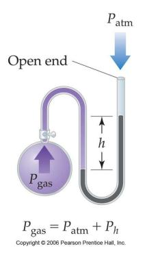
We know that this pressure must be greater than atmospheric because the manometer level on the flask side (103.8 mm) is lower than that on the side open to the atmosphere (136.4 mm), as indicated in Figure
