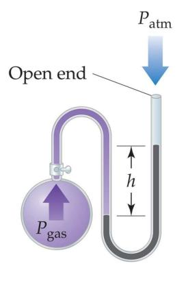
Used to measure the difference in pressure between atmospheric pressure and that of a gas in a vessel.
