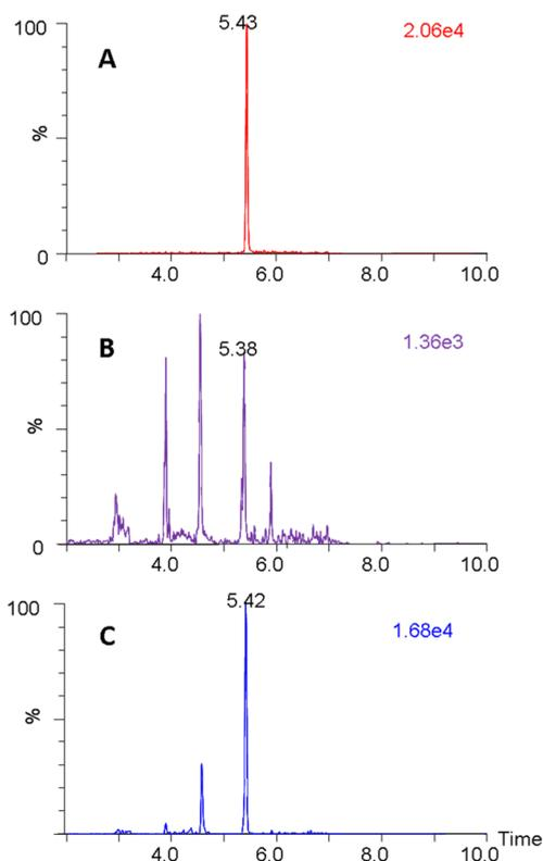
**Figure 3.** Extracted ion chromatograms of thiazolidine-4-carboxylic acid derivative ( $m/z$  206.0–206.1) obtained from UPLC-MS analyses of (A) blank PBS spiked with 1 ng/mL thiazolidine-4-carboxylic acid, (B) untreated *E. coli*, and (C) *E. coli* treated with 2.5 mM Fe<sup>2+</sup>-EDTA.
