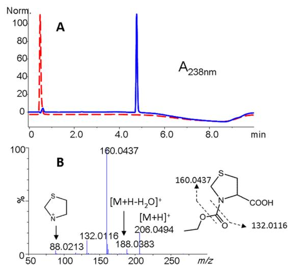
**Figure 1.** (A) Chromatograms obtained from reversed-phase HPLC analysis of thiazolidine-4-carboxylic acid (dashed red line) and 3-(ethoxycarbonyl)thiazolidine-4-carboxylic acid (solid blue line). (B) ESI–MS/MS spectrum of the pseudomolecular ion  $[\text{M} + \text{H}]^+$  ion of 3-(ethoxycarbonyl)thiazolidine-4-carboxylic acid at  $m/z$  206 and the cleavage reactions for the formation of major fragment ions found in MS/MS analysis.
