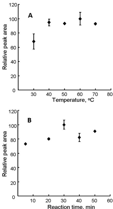
**Figure 2.** Influence of (A) temperature and (B) time on the yield of the derivatization reaction. The data represent the mean  $\pm$  SD of three independent experiments.
